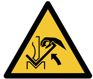
ISO 7010 W031 Warning; Hand crushing between press brake and material
